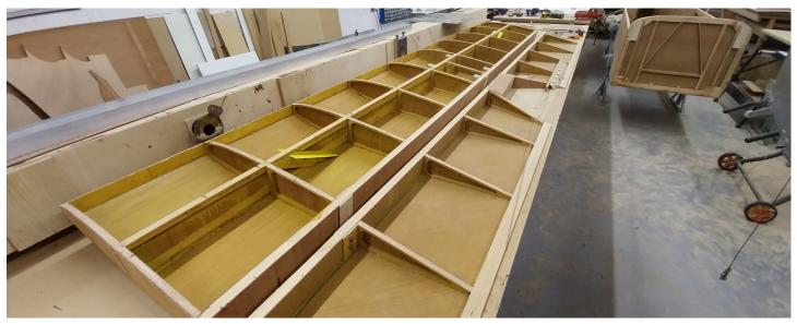
A wing before skinning with plywood showing its simple but strong design. So, what engine & propeller will Chris fit to this racy aircraft? "Oh that's some way down the line, so I haven't decided yet". We will wait with bated breath to see this beast at PF sometime in the future.
