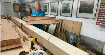
It is a plans-built aircraft, not a kit. That beefy main spar has to take the retractable landing gear, but the wing ribs are a bit different and very light. You need a fairly large workshop to build an aircraft like this one - fortunately Chris has such a facility.
